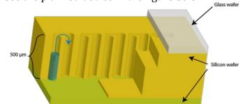
Figure: 3D-Drawing of the planned microfluidic device: holes of different diameters etched through the wafer with connection channels at top and bottom. To close the device, a silicon wafer will be bonded on the bottom and (for optical access) a glass wafer on the top.
